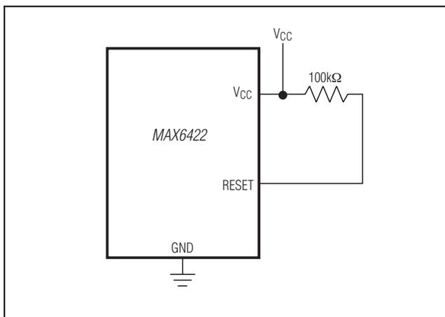
Figure 4. Ensuring  $\overline{\text{RESET}}$  Valid to  $V_{\text{CC}} = 0$
