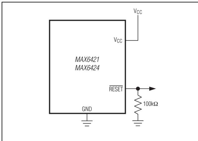
Figure 3. Ensuring  $\overline{\text{RESET}}$  Valid to  $V_{\text{CC}} = 0$
