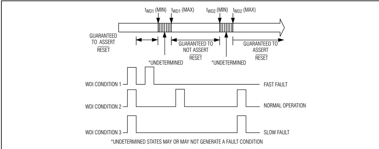
Figure 1. MAX6752/MAX6753 Detailed Watchdog Input Timing Relationship
