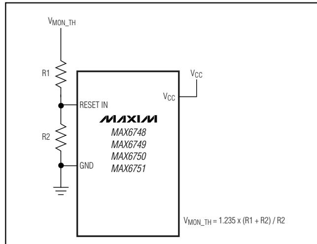
Figure 2. Calculating the Monitored Threshold Voltage (V<sub>MON\_TH</sub>)
