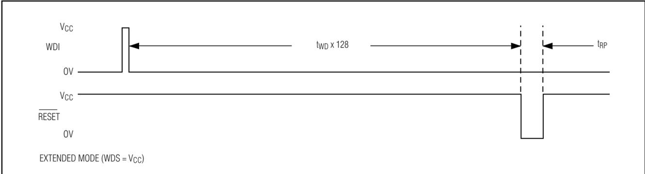
Figure 4b. Watchdog Timing Diagram, WDS = VCC
