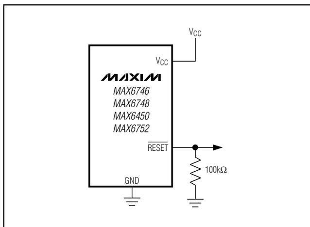
Figure 7. Ensuring  $\overline{\text{RESET}}$  Valid to  $V_{CC} = 0$
