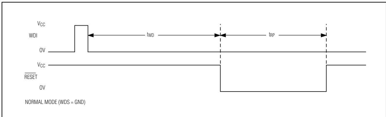
Figure 4a. Watchdog Timing Diagram, WDS = GND
