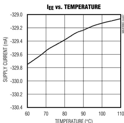
DUT<sub>-</sub> = DTV<sub>-</sub> = 1.5V, DHV<sub>-</sub> = 3V, DLV<sub>-</sub> = 0, CHV<sub>-</sub> = CLV<sub>-</sub> = 0, CPHV<sub>-</sub> = 7.2V, CPLV<sub>-</sub> = -2.2V, V<sub>CC</sub> = 9.75V, V<sub>EE</sub> = -5.25V
