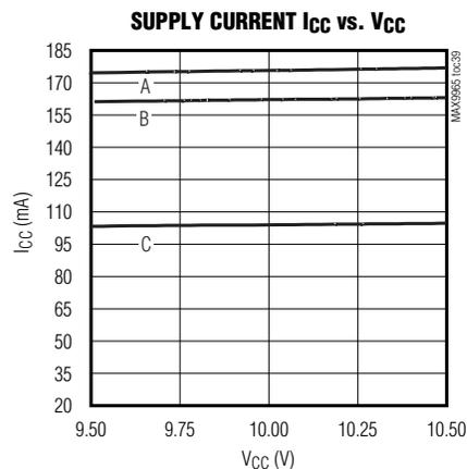
A: DUT<sub>-</sub> = DTV<sub>-</sub> = 1.5V, DHV<sub>-</sub> = 3V, DLV<sub>-</sub> = 0, CHV<sub>-</sub> = CLV<sub>-</sub> = 0, CPHV<sub>-</sub> = 7.2V, CPLV<sub>-</sub> = -2.2V
