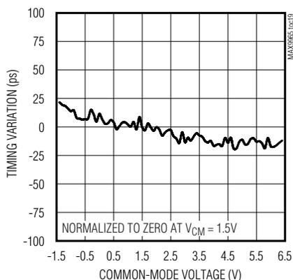
**COMPARATOR FALLING EDGE TIMING VARIATION vs. COMMON-MODE VOLTAGE**
