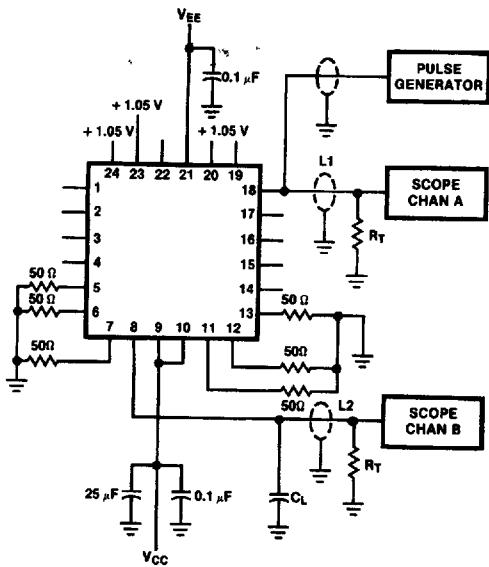
**Notes:** $V_{CC}, V_{CCA} = +2V, V_{EE} = -2.5V$ L<sub>1</sub> and L<sub>2</sub> = equal length 50Ω impedance linesR<sub>T</sub> = 50Ω terminator internal to scopeDecoupling 0.1 μF from GND to  $V_{CC}$  and  $V_{EE}$
