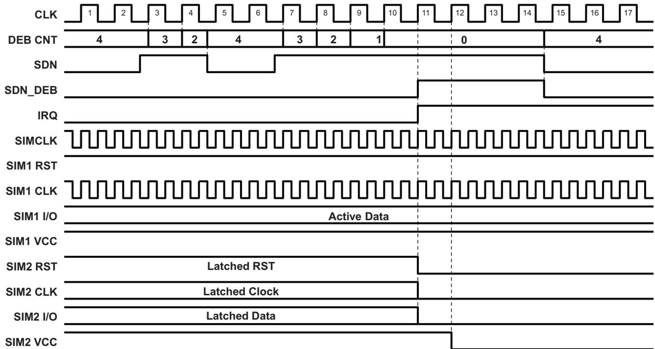
Figure 6. SDN Debounce Timing – SDN Detection Level High
