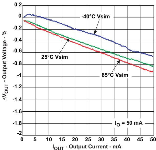
Figure 14. Load Regulation, Iout = 50 mA, Class-B
