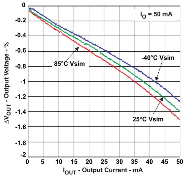
Figure 13. Load Regulation, Iout = 50 mA, Class-C
