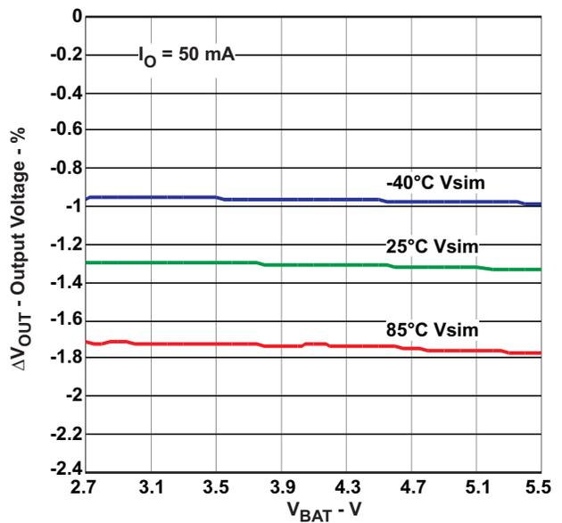
Figure 15. Line Regulation, Iout = 50 mA, Class-C
