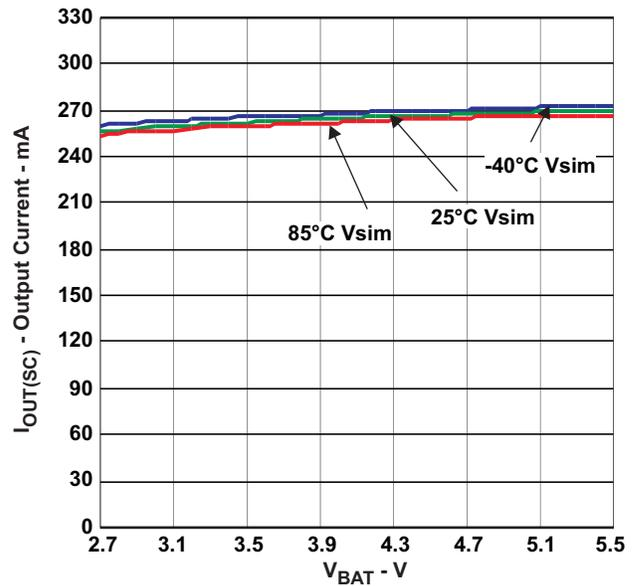
Figure 17. Current Limit vs Input Voltage, Class-B/C
