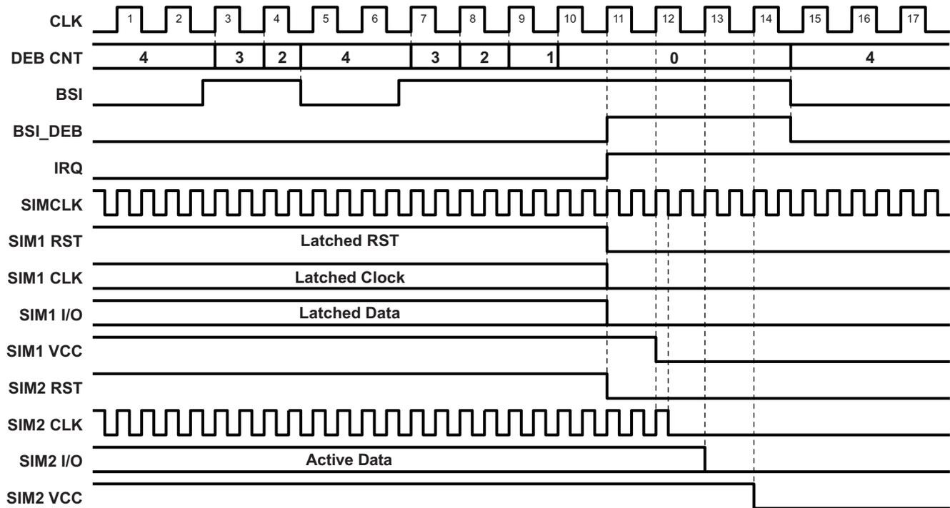
Figure 4. BSI Debounce Timing – SIM1 Isolated, SIM2 Active
