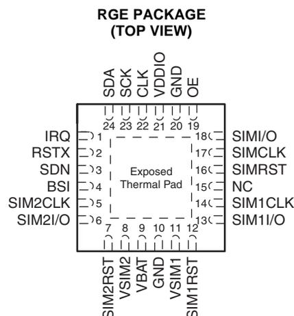
Note: The Exposed Thermal Pad must be connect to Ground.
