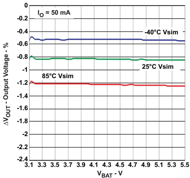
Figure 16. Line Regulation, I<sub>out</sub> = 50 mA, Class-B
