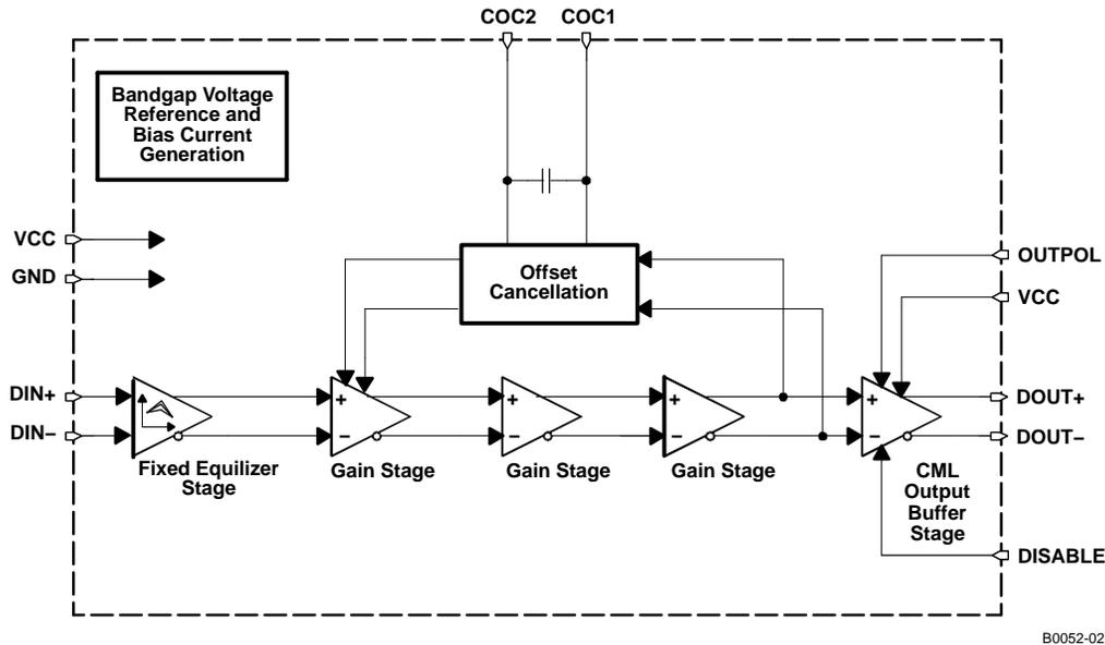
**Figure 1. Simplified Block Diagram of the TLK4211EA**
