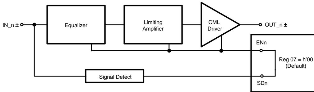
Figure 10. Automatic Enable Configuration
