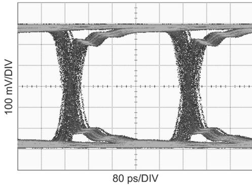
**Figure 11. Equalized Signal**
