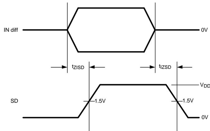
Figure 5. Signal Detect (SD) Delay Timing Diagram
