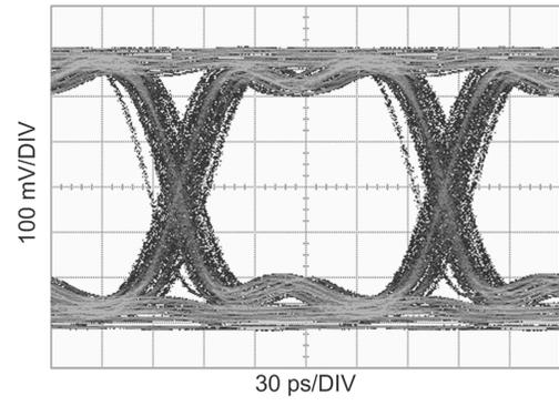
**Figure 16. Equalized Signal**
