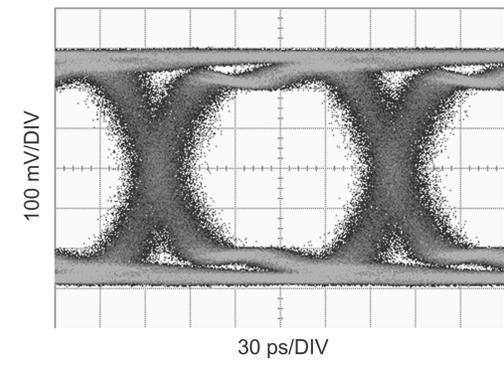
**Figure 14. Equalized Signal**
