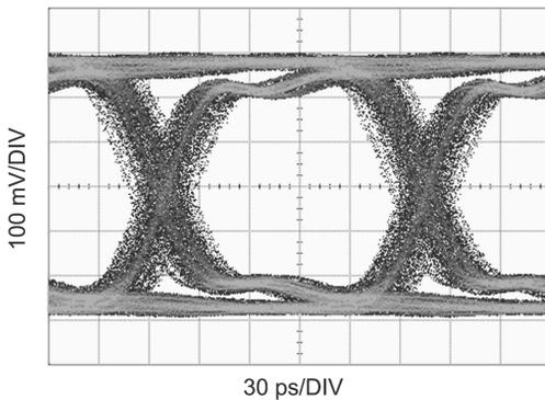
**Figure 13. Equalized Signal**
