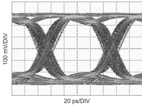
**Figure 15. Equalized Signal**
