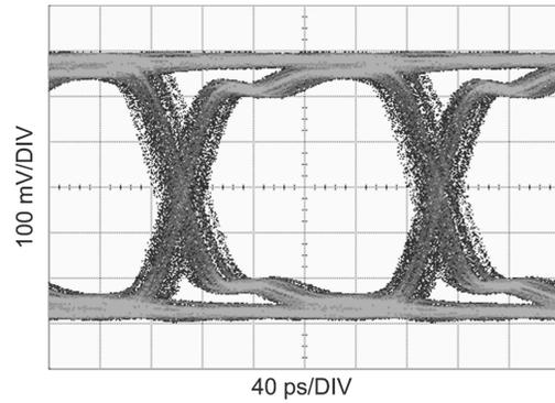
**Figure 12. Equalized Signal**
