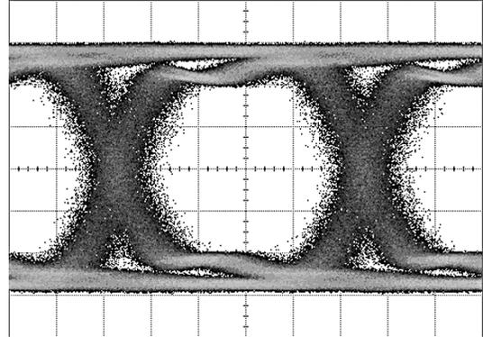
**Figure 10. Equalized Signal
