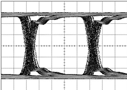
**Figure 7. Equalized Signal**
