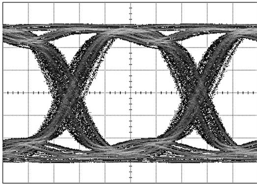
**Figure 11. Equalized Signal
