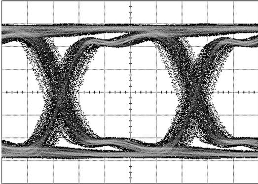
**Figure 9. Equalized Signal
