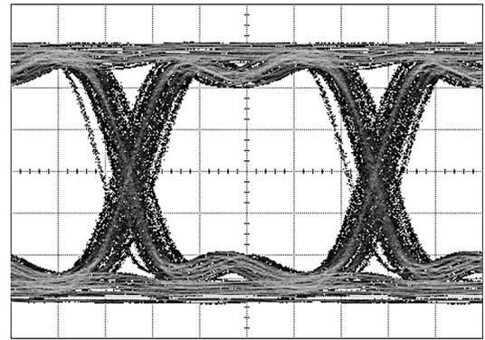
**Figure 12. Equalized Signal
