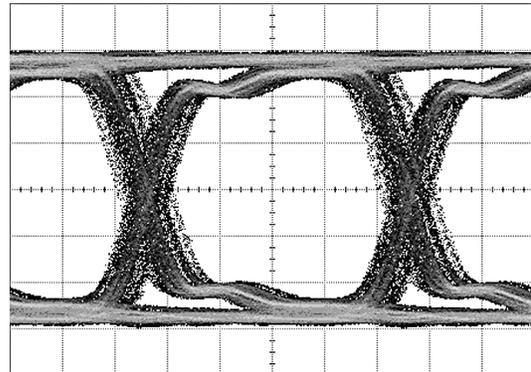
**Figure 8. Equalized Signal**
