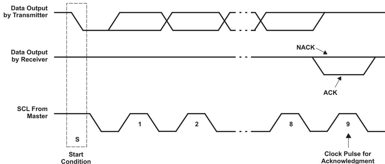
**Figure 7. Acknowledgment on I<sup>2</sup>C Bus**
