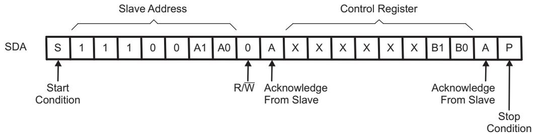
Figure 8. Write Control Register
