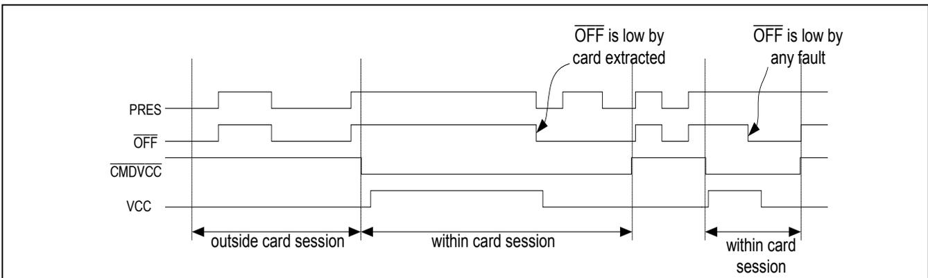
Figure 9: Timing Diagram—Management of the Interrupt Line  $\overline{\text{OFF}}$
