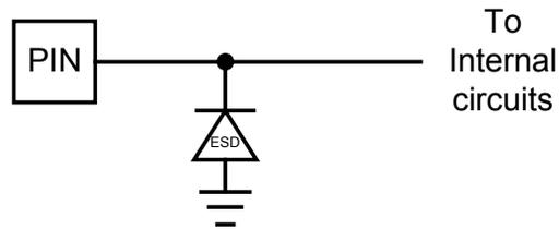
Figure 13: Power Input/Output Circuit— $V_{DD}$ ,  $V_{PC}$ ,  $V_{CC}$
