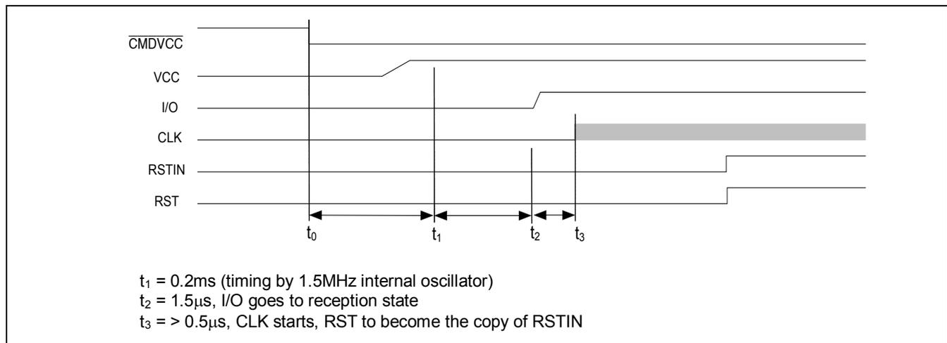
**Figure 6: Activation Sequence—RSTIN Low When  $\overline{CMDVCC}$  Goes Low**
