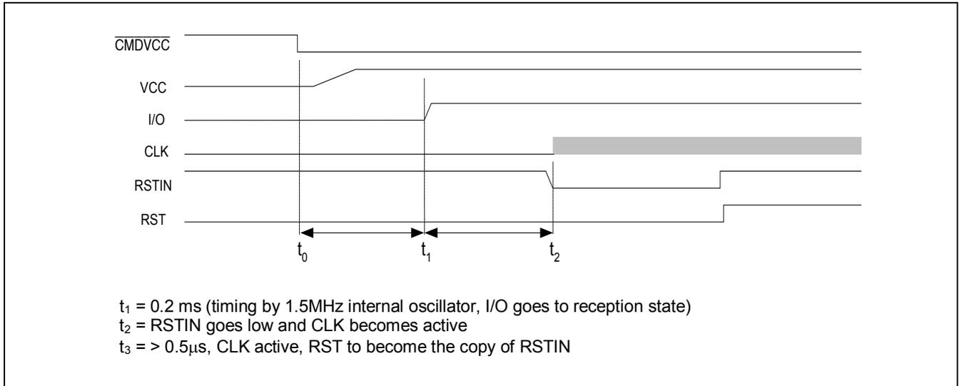
**Figure 7: Activation Sequence—RSTIN High When  $\overline{\text{CMDVCC}}$  Goes Low**
