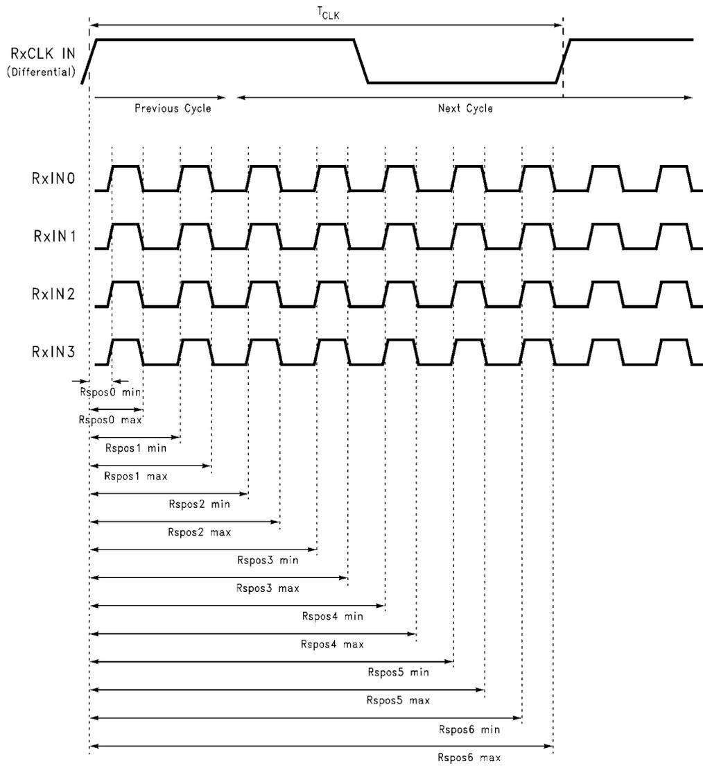
FIGURE 9. DS90CR286A (Receiver) LVDS Input Strobe Position
