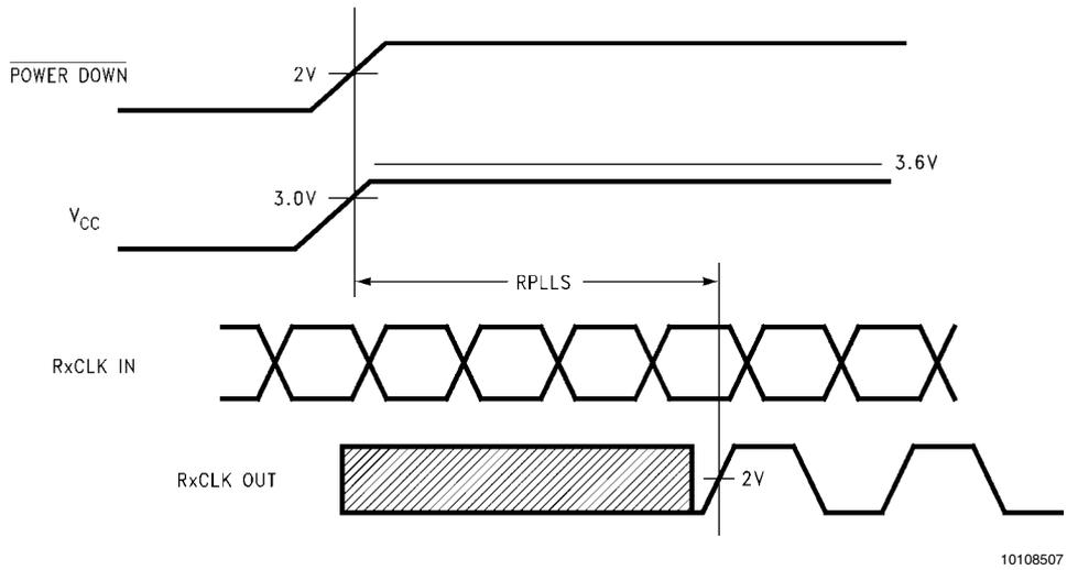
FIGURE 7. DS90CF386/DS90CF366 (Receiver) Phase Lock Loop Set Time
