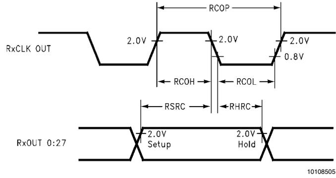
FIGURE 5. DS90CF386/DS90CF366 (Receiver) Setup/Hold and High/Low Times
