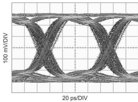
**Figure 12. Equalized Signal**
