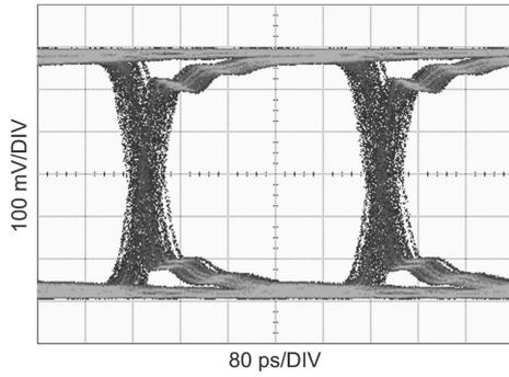
**Figure 8. Equalized Signal**
