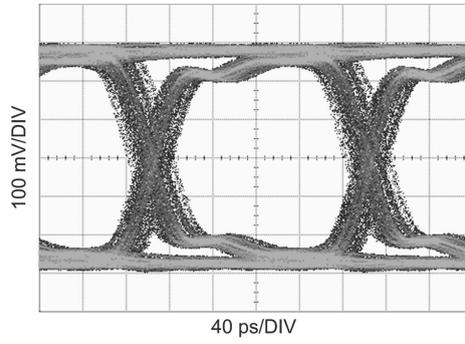
**Figure 9. Equalized Signal**
