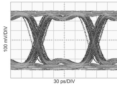
**Figure 13. Equalized Signal**
