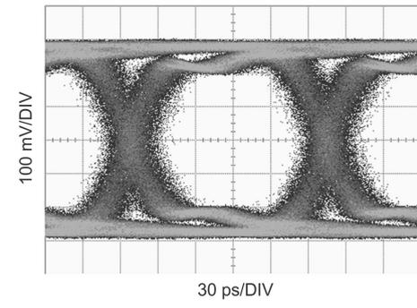
**Figure 11. Equalized Signal**
