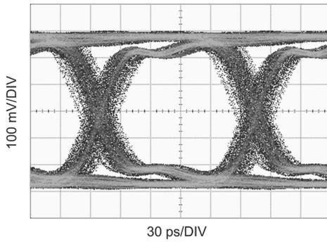
**Figure 10. Equalized Signal**
