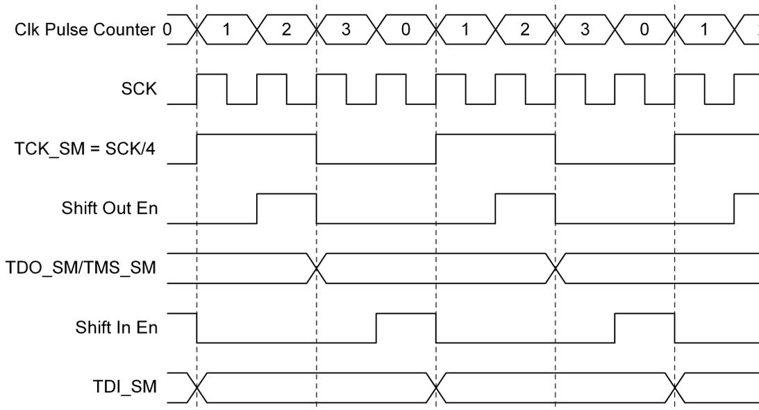
**Figure 6. Shift Register Implementation and Timing**
