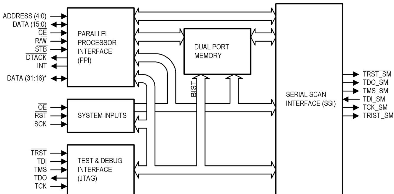
\* Note: IP data bus width can be configured for 16 or 32 bit applications. Silicon data bus width is fixed at 16 bits.
