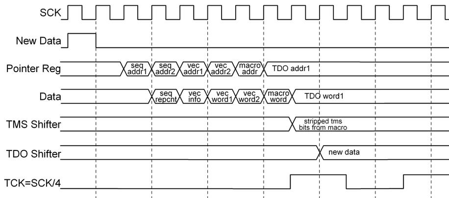
**Figure 9. Timing from Mode Register to Sequencer Start**
