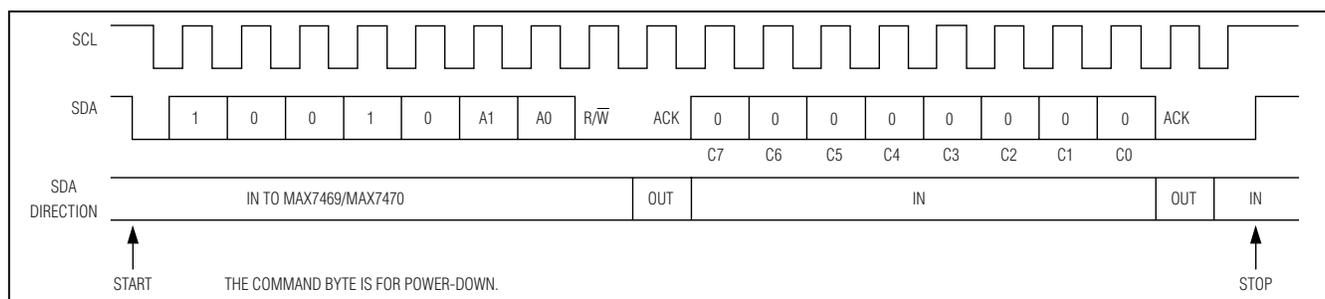
Figure 7. Write Sequence for a Command Byte
