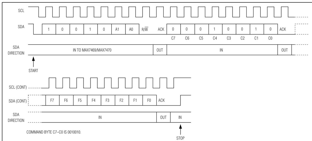
Figure 6. Write Sequence to Update the Frequency Register
