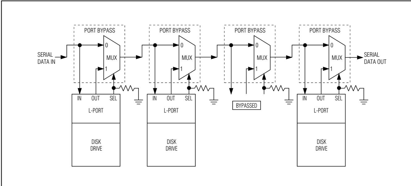
Figure 2. Disk Array Implemented with Port Bypass Circuits
