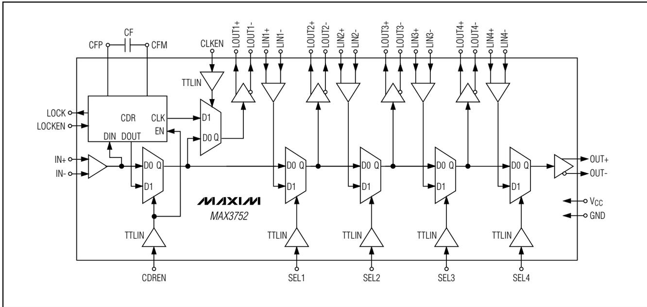
Figure 1. Functional Diagram
