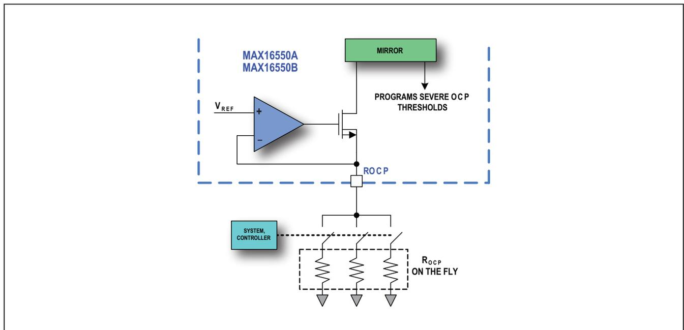
Figure 4. On-The-Fly Analog Programmable Moderate OCP Threshold
