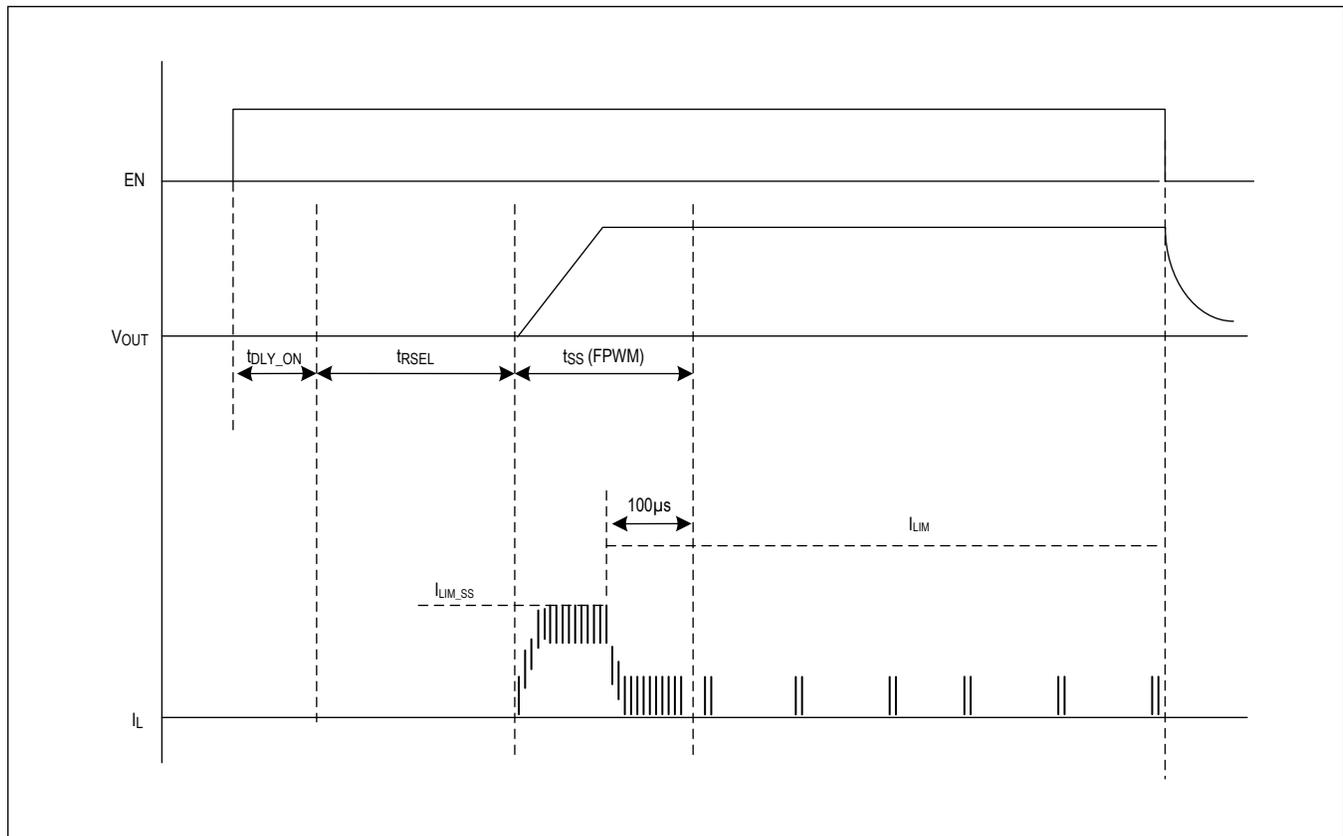
Figure 1. Startup Waveform
