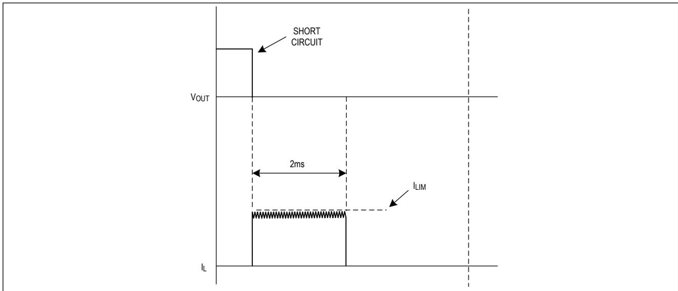
Figure 2. Short-Circuit Waveform
