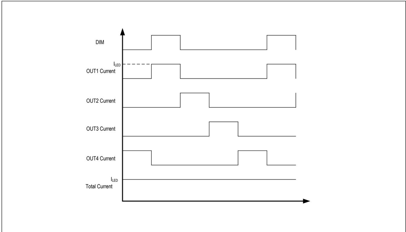
Figure 2. Phase-Shifted Outputs
