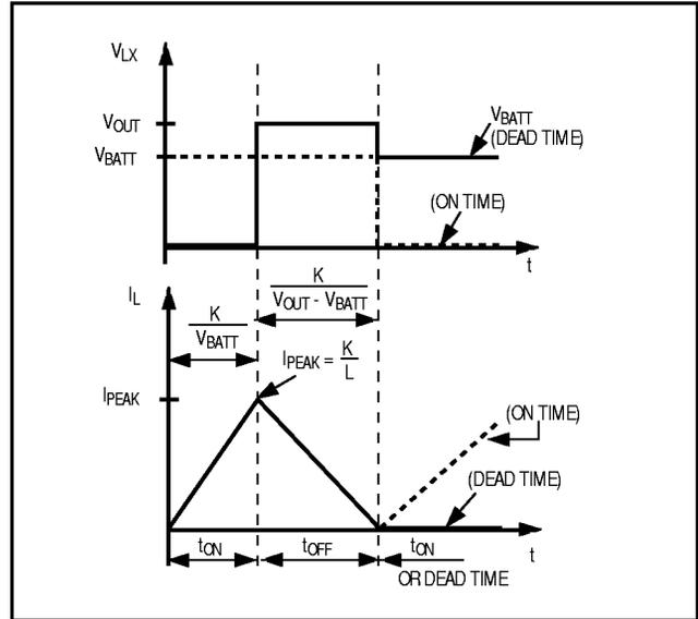
Figure 2. Switching Waveforms
