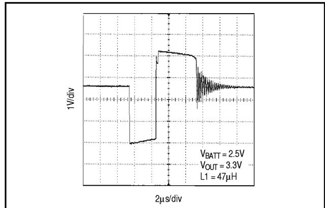
Figure 5. LX Ringing Without Damping Switch (example only)
