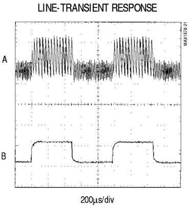
$V_{OUT} = 3.3\text{V}$ ,  $V_{BATT} = 1.2\text{V}$ ,  $I_{LOAD} = 10\text{mA}$ ,  $C_{OUT} = 10\mu\text{F}$ ,  $L1 = \text{SUMIDA CD43-470}$
