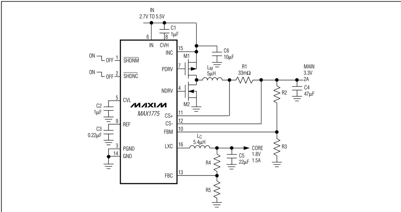
Figure 1. Typical Application Circuit (Low Input Voltage)
