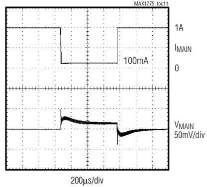
**MAIN LOAD TRANSIENT (IN DROPOUT)
