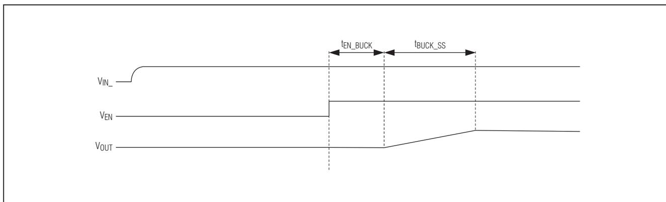
Figure 2. Power-Up Timing
