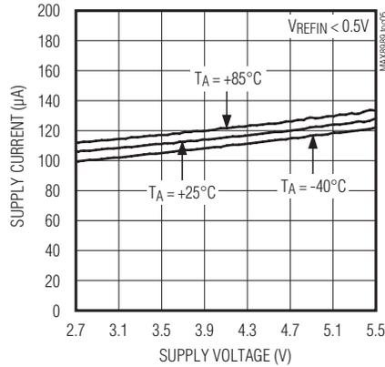
**NO LOAD SUPPLY CURRENT vs. SUPPLY VOLTAGE (FPWM MODE)**
