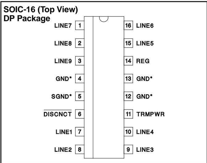
\* DP package pin 5 serves as signal ground; pins 4, 12, 13 serve as heatsink/ground.
