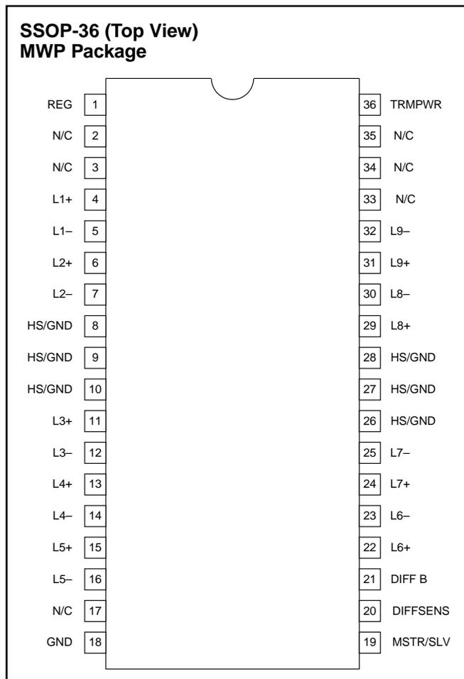
**ELECTRICAL CHARACTERISTICS:** Unless otherwise specified, TA = 0°C to 70°C, TRMPWR = 3.3V.
