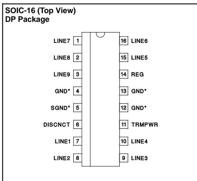
\* DP package pin 5 serves as signal ground; pins 4, 12, 13 serve as heatsink/ground.
