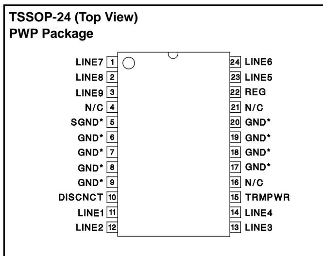
\* PWP package pin 5 serves as signal ground; pins 6, 7, 8, 9, 17, 18, 19, and 20 serve as heatsink/ground.
