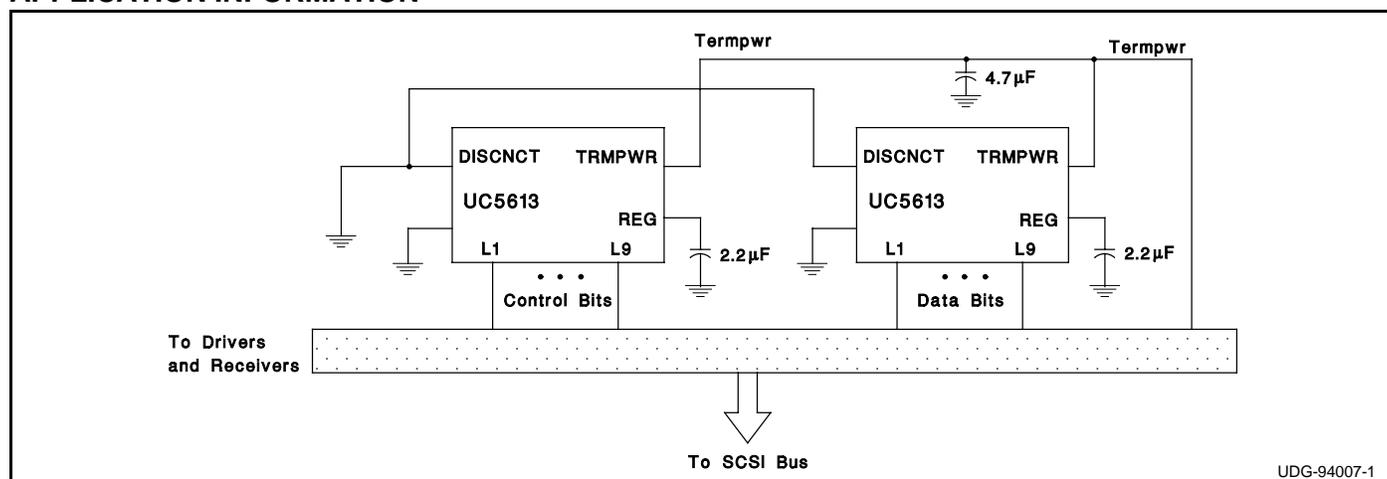
Figure 1: Typical SCSI Bus Configurations Utilizing 2 UC5613 Devices
