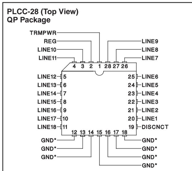
\* DWP package pins 12-18 serve as both heatsink and signal ground.
