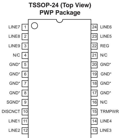
\* PWP package pin 9 serves as signal ground; pins 5, 6, 7, 8, 17, 18, 19 and 20 serve as heatsink/ground.
