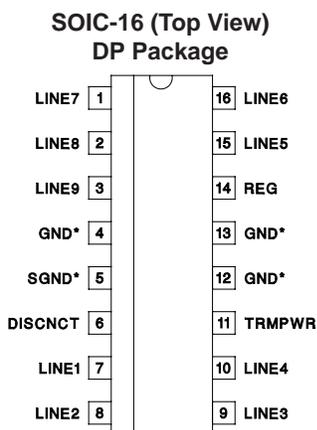
\* DP package pin 5 serves as signal ground; pins 4, 12, and 13 serve as heatsink/ground.
