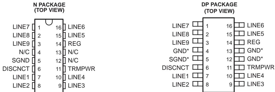
\* DP package pin 5 serves as signal ground; pins 4, 12, 13 serve as heatsink/ground.
