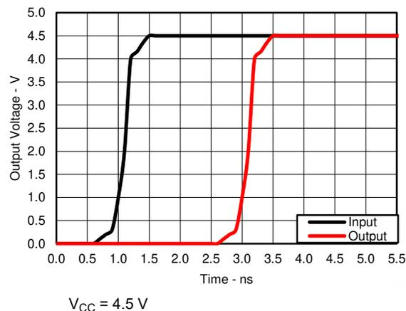
Figure 10-2. Propagation Delay ( $t_{pd}$ ) Simulation Results
