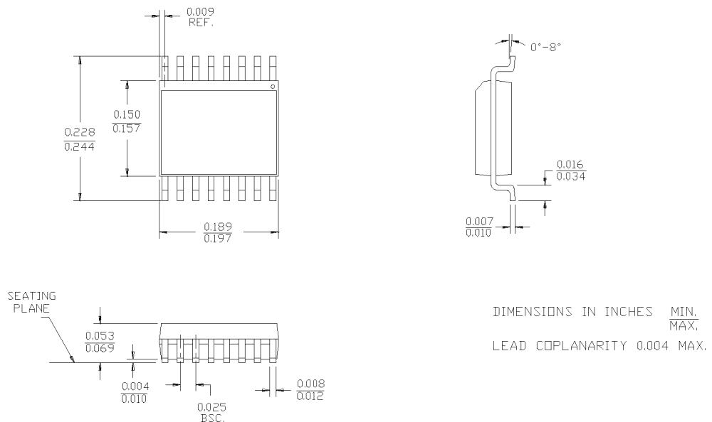
**16-Lead Molded SOIC S1**
