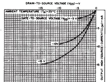
Fig. 6 - Minimum output high (source) current characteristics.
