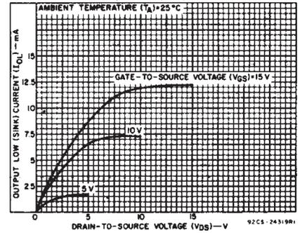
Fig. 4 - Minimum output low (sink) current characteristics.
