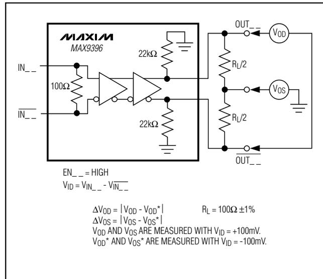
Figure 2. Test Circuit for VOD and VOS
