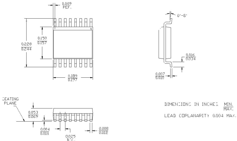
**16-Lead Molded SOIC S1**
