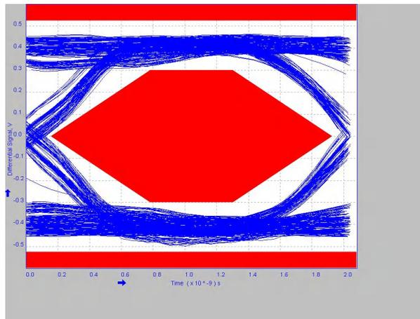
Figure 7-7. 5 Meter Pre-Channel With TUSB211A-Q1 EQ=2
