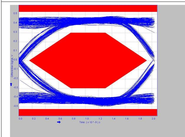
Figure 5-3. 2 Meter Post-Channel With TUSB211A-Q1 EQ=1
