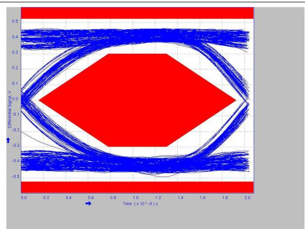
Figure 7-14. 4 Meter Post-Channel With TUSB211A-Q1 EQ=2
