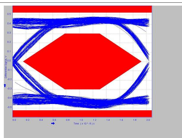
Figure 7-4. 2 Meter Pre-Channel With TUSB211A-Q1 EQ=1
