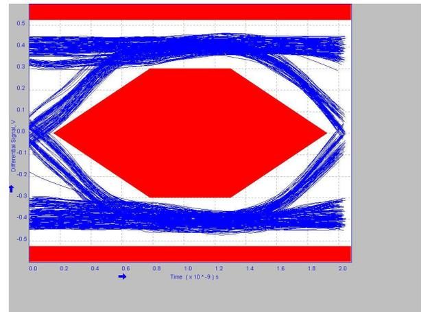
Figure 7-6. 5 Meter Pre-Channel With TUSB211A-Q1 EQ=1
