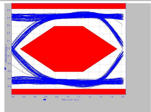
Figure 7-10. 1 Meter Post-Channel With TUSB211A-Q1 EQ=0
