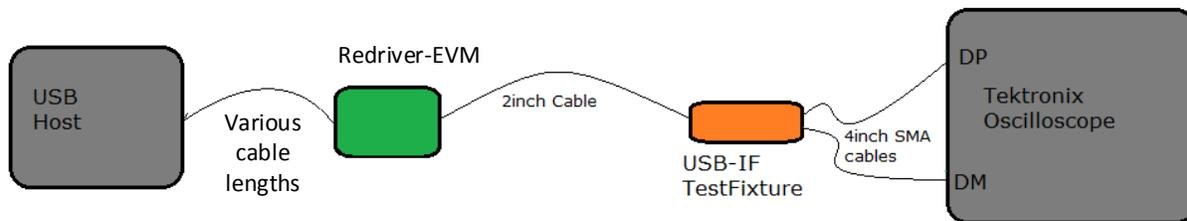
Figure 7-2. Near End Eye Measurement Set-Up With Pre-Channel Cable
