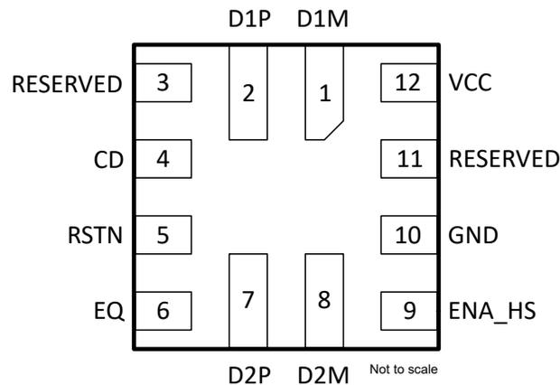
Figure 4-1. TUSB211A-Q1 RWB 12-Pin X2QFN (Top View)
