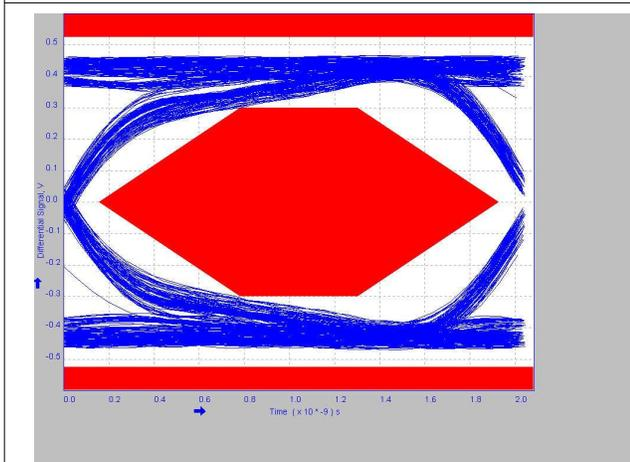
Figure 7-11. 2 Meter Post-Channel Without TUSB211A-Q1
