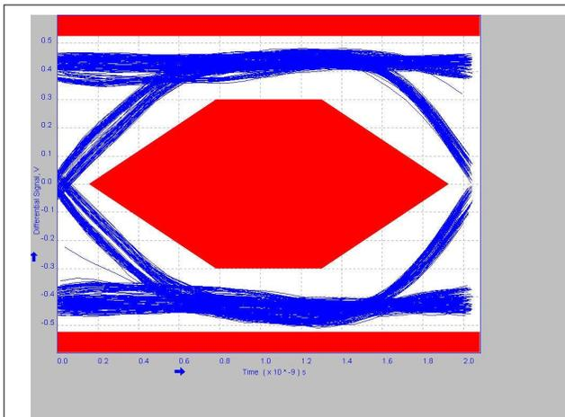
Figure 5-1. 2 Meter Pre-Channel With TUSB211A-Q1 EQ=1
