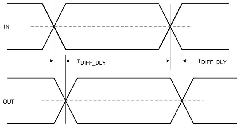
Figure 6-3. Propagation Delay
