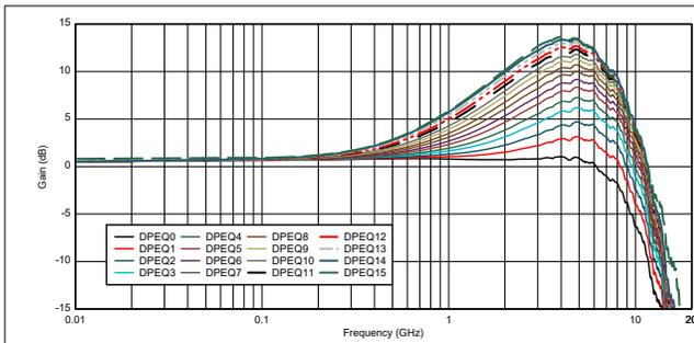
Figure 5-1. DisplayPort EQ Settings Curves at Nominal Conditions
