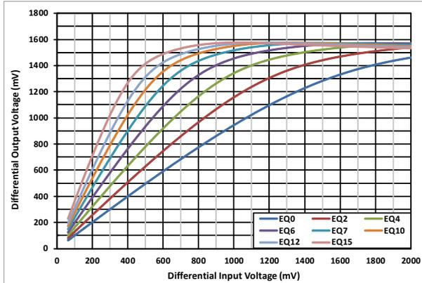
**Figure 5-9. USB RX (UFP) Linearity Curves at 2.5GHz**
