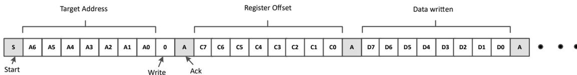
**Figure 7-2. I<sup>2</sup>C Write with Data**
