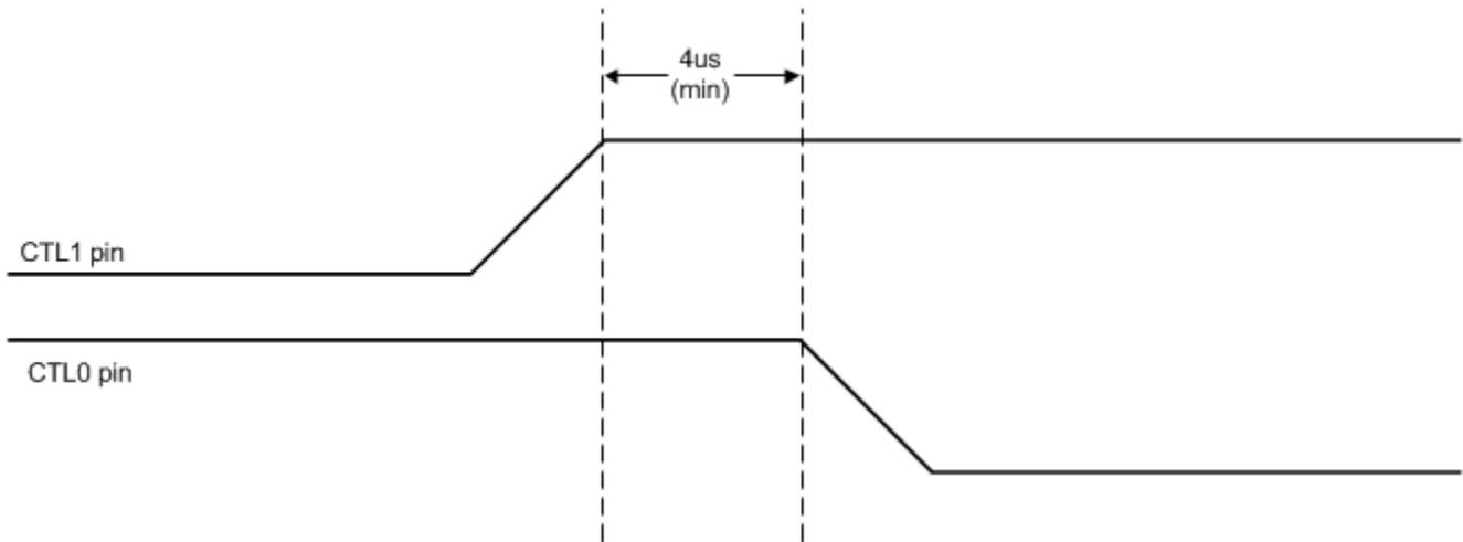
Figure 6-2. USB3.1 to 4-Lane DisplayPort in GPIO Mode
