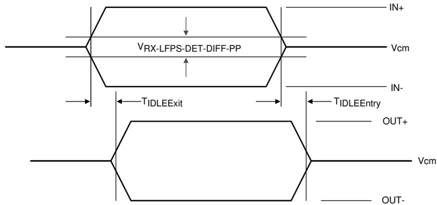
**Figure 6-4. Electrical Idle Mode Exit and Entry Delay**
