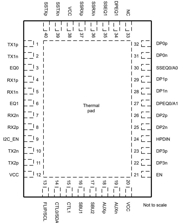
**Figure 4-1. RGF Package, 40-Pin (VQFN) (Top View)**
