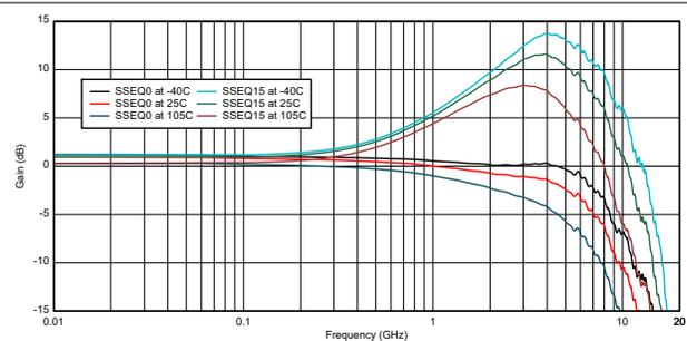
Figure 5-6. USB3 SSTX SSEQ0 and SSEQ15 Across Temperature
