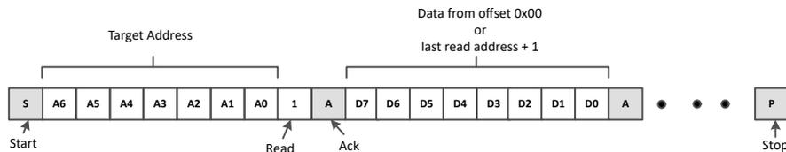
**Figure 7-3. I<sup>2</sup>C Read Without Repeated Start**
