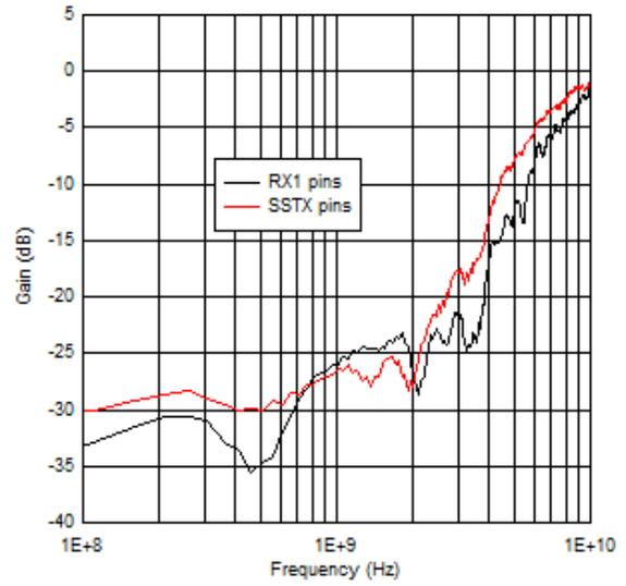
**Figure 5-10. Input Return Loss Performance**
