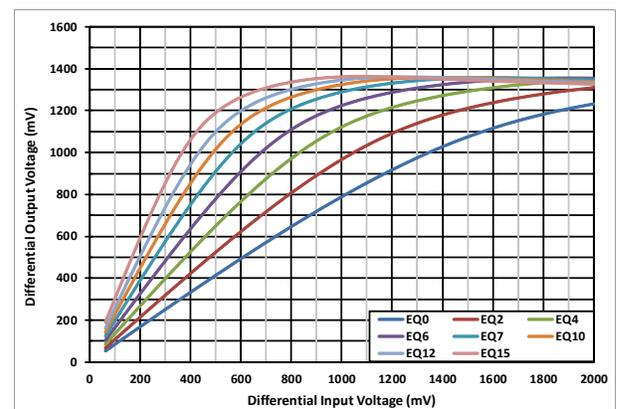
Figure 5-8. USB TX (DFP) Linearity Curves at 2.5GHz
