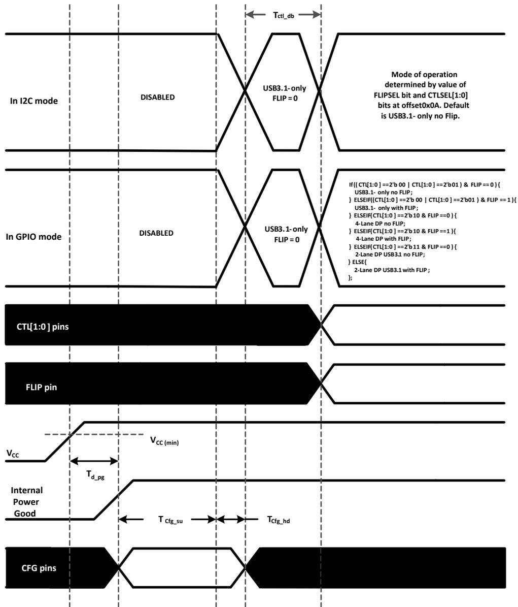
Figure 7-1. Power-Up Timing
