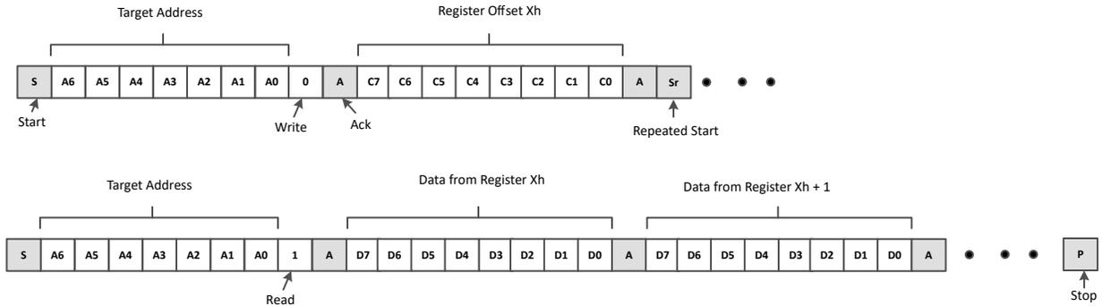
**Figure 7-4. I<sup>2</sup>C Read with Repeated Start**
