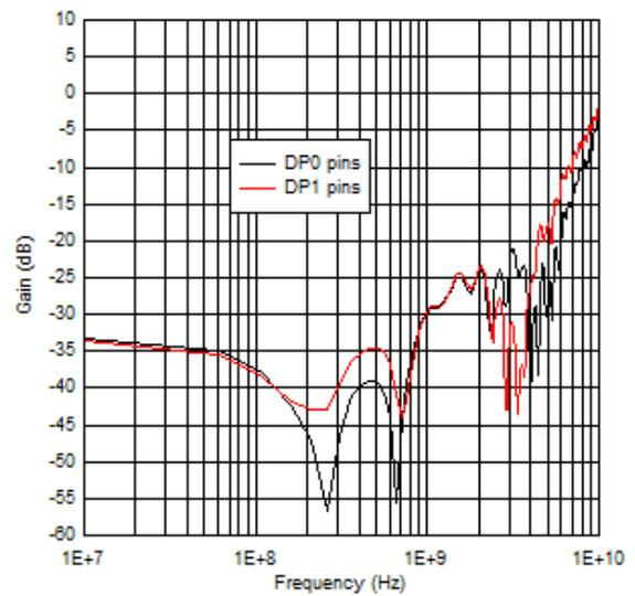
**Figure 5-12. DisplayPort Output Return Loss Performance**
