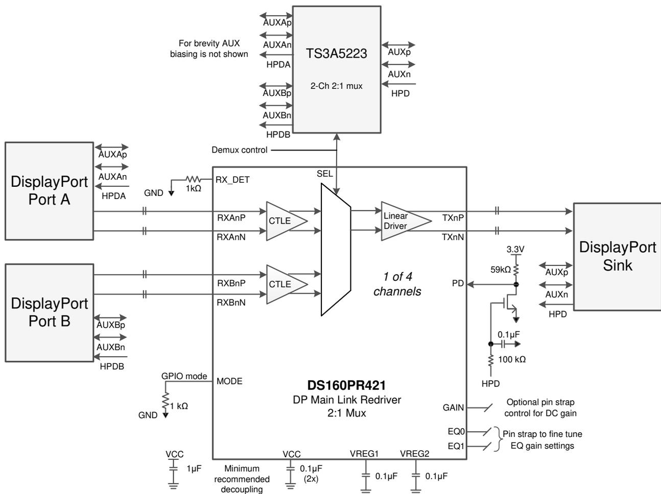
Figure 8-4. Simplified Schematic for DisplayPort Multiplexer Application
