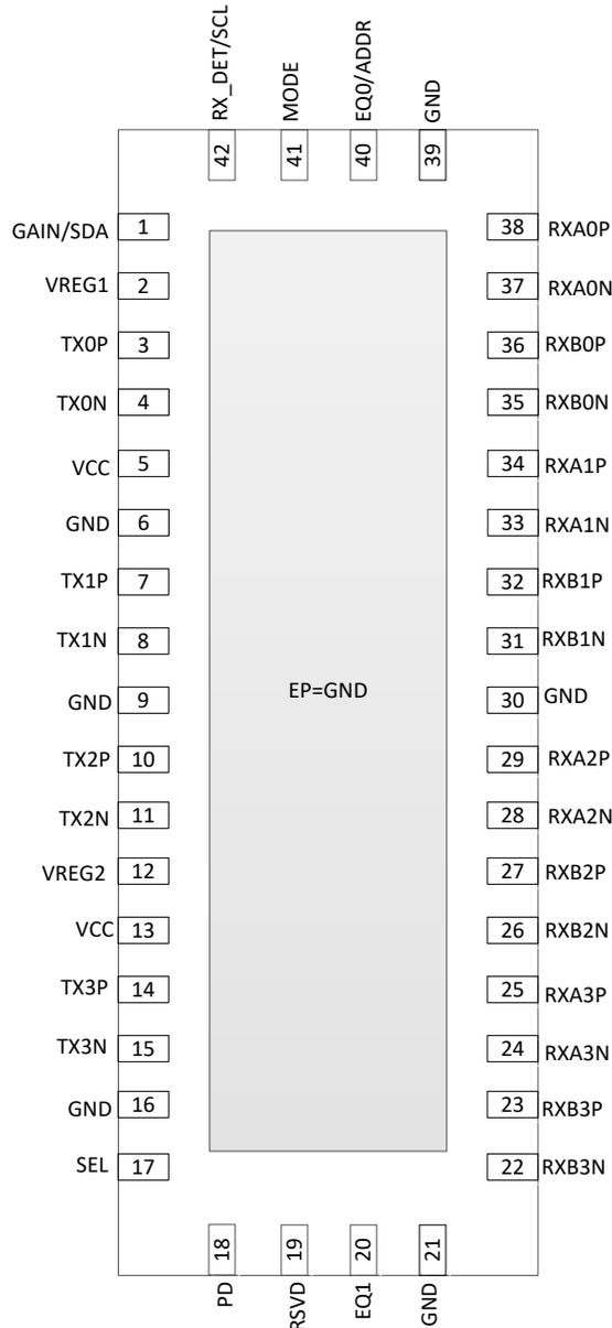
**Figure 5-1. RUA Package 42-Pin WQFN Top View**
