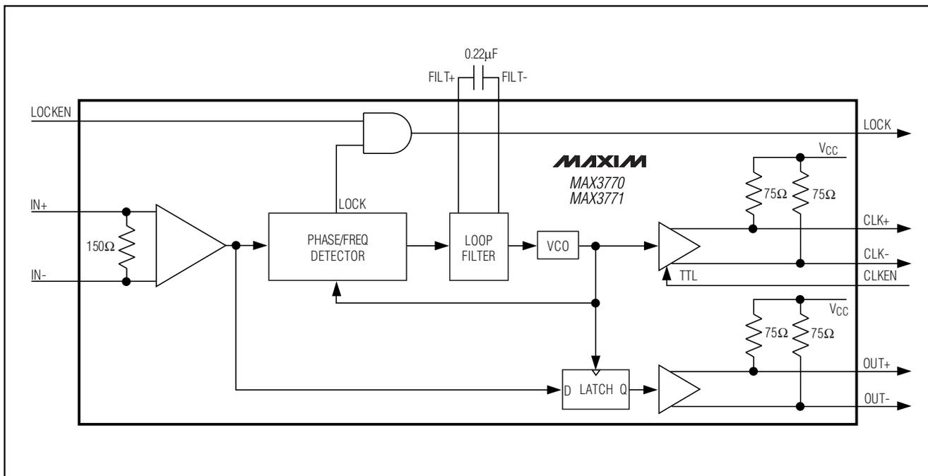
Figure 2. Functional Diagram
