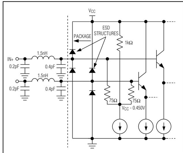
Figure 3. Input Structure
