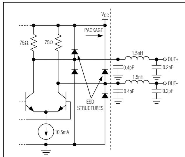
Figure 4. Output Structure
