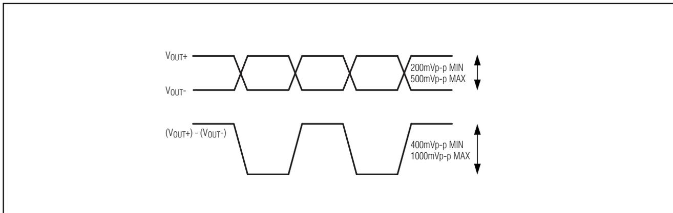
Figure 1. Example of Output Signal with  $R_{LOAD} = 150\Omega$
