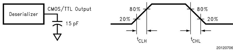
FIGURE 5. Deserializer CMOS/TTL Output Load and Transition Times
