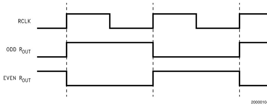
FIGURE 3. "Worst Case" Deserializer ICC Test Pattern
