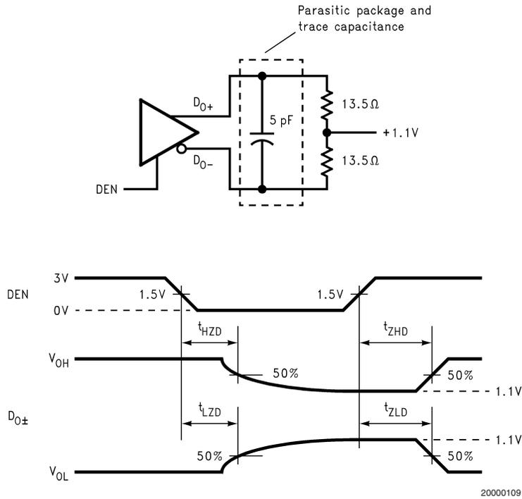
FIGURE 8. Serializer TRI-STATE Test Circuit and Timing
