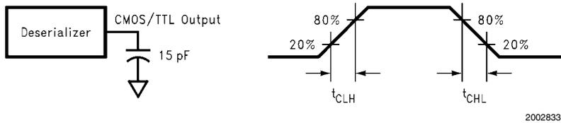
**FIGURE 3. Deserializer CMOS/LVTTL Output Load and Transition Times**
