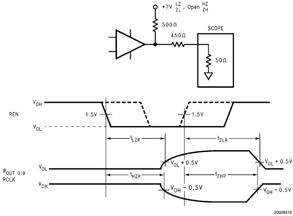
FIGURE 7. Deserializer TRI-STATE Test Circuit and Timing
