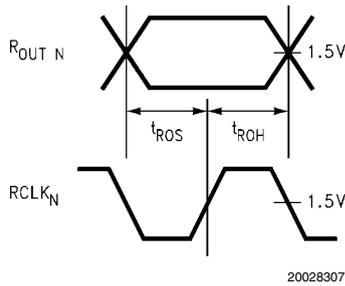
**FIGURE 2. Output Timing  $t_{ROS}$  and  $t_{ROH}$  (Data Valid)**
