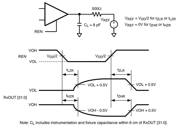
Figure 12. Deserializer TRI\_STATE Test Circuit and Timing
