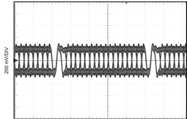
**Figure 21. Serial Output, 50 MHz, VSEL = L,
