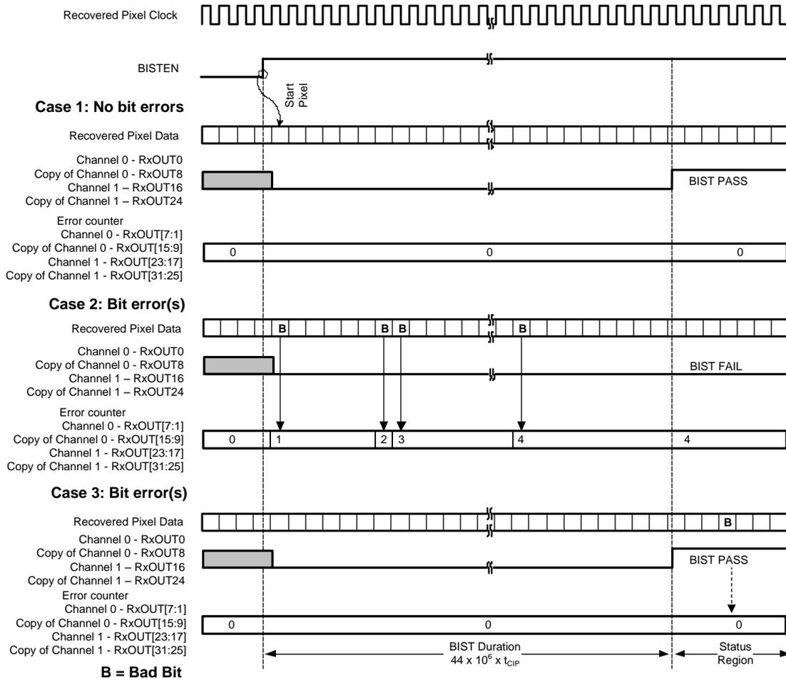
Figure 17. BIST Diagram for Different Bit Error Cases
