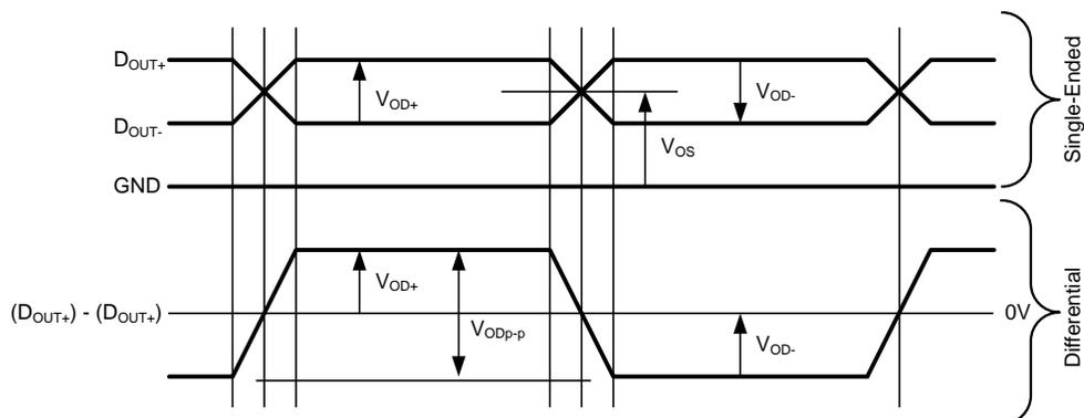
Figure 3. Output Waveforms
