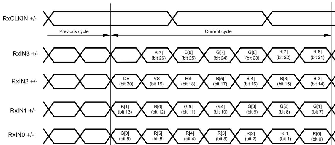
**Figure 17. 8-Bit FPD-Link Mapping: MSB's on Rxin3**
