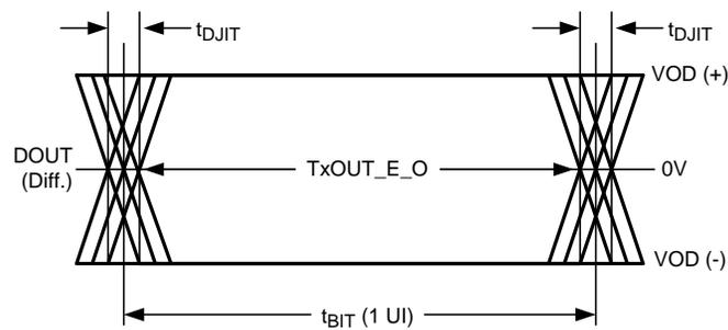
Figure 9. Output Jitter
