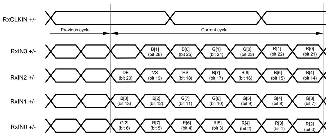
Figure 16. 8-Bit FPD-Link Mapping: LSB's on Rxin3
