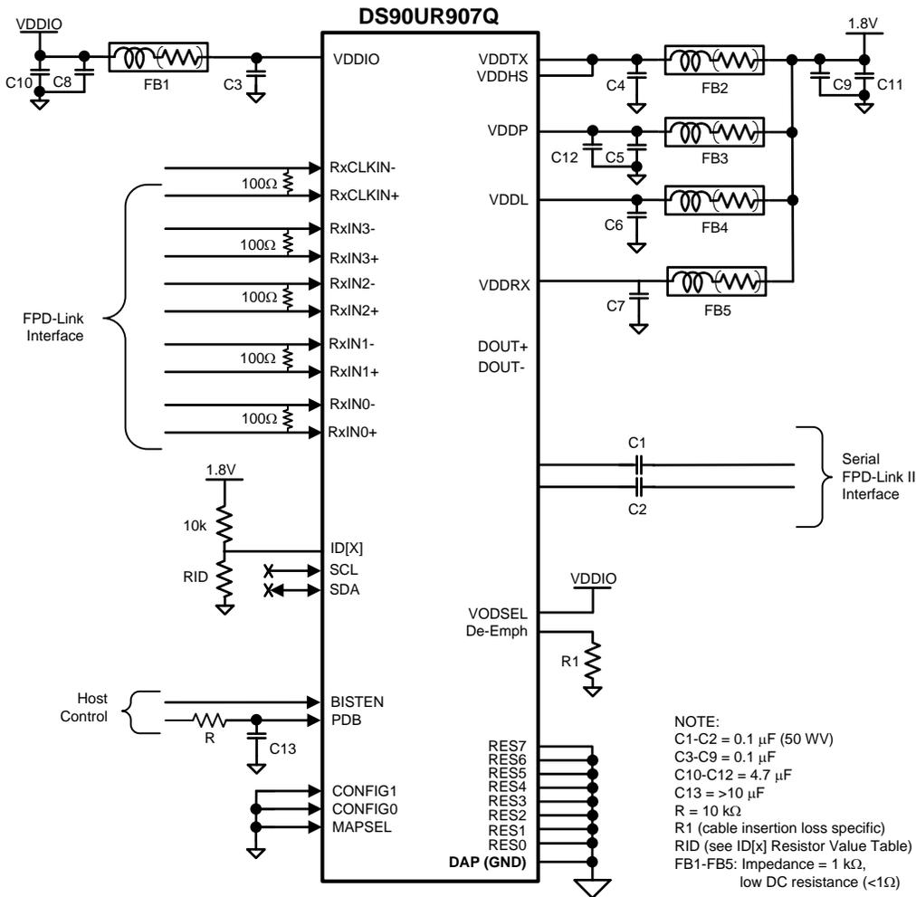
Figure 25. Typical Connection Diagram
