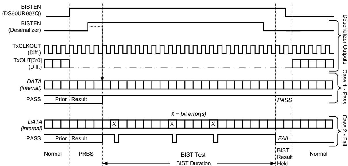
**Figure 20. BIST Waveforms**
