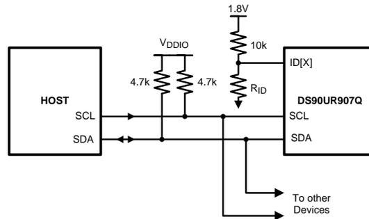
Figure 21. Serial Control Bus Connection
