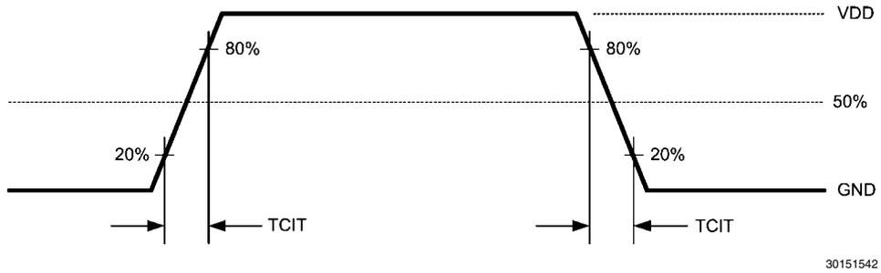
FIGURE 5. DS90C185 (Transmitter) Input Clock Transition Time
