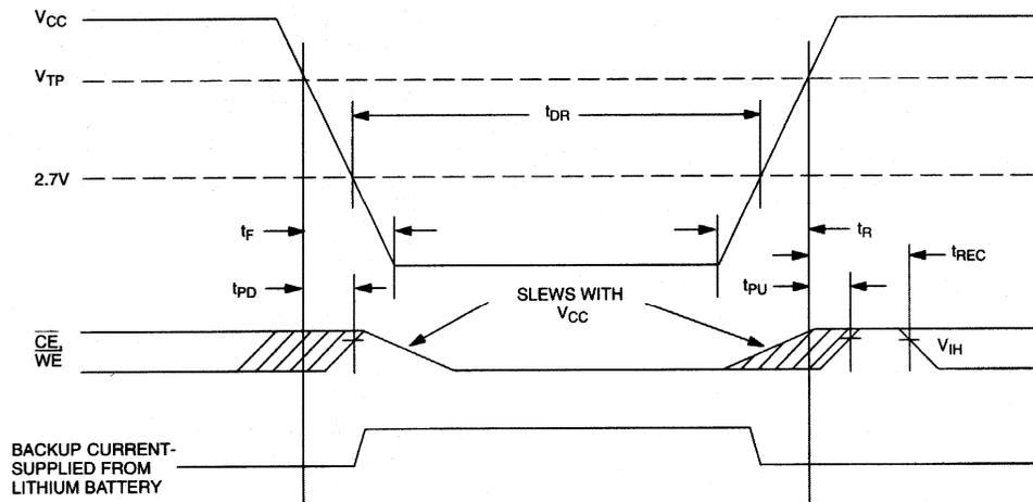
**POWER-DOWN/POWER-UP TIMING**(t<sub>A</sub>: See Note 10)
