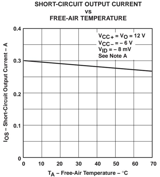
NOTE A: This parameter was measured using a single 5-ms pulse.
