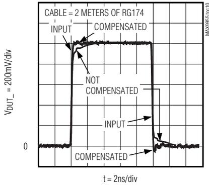
**COMPARATOR WAVEFORM TRACKING WITHOUT CABLE COMPENSATION**
