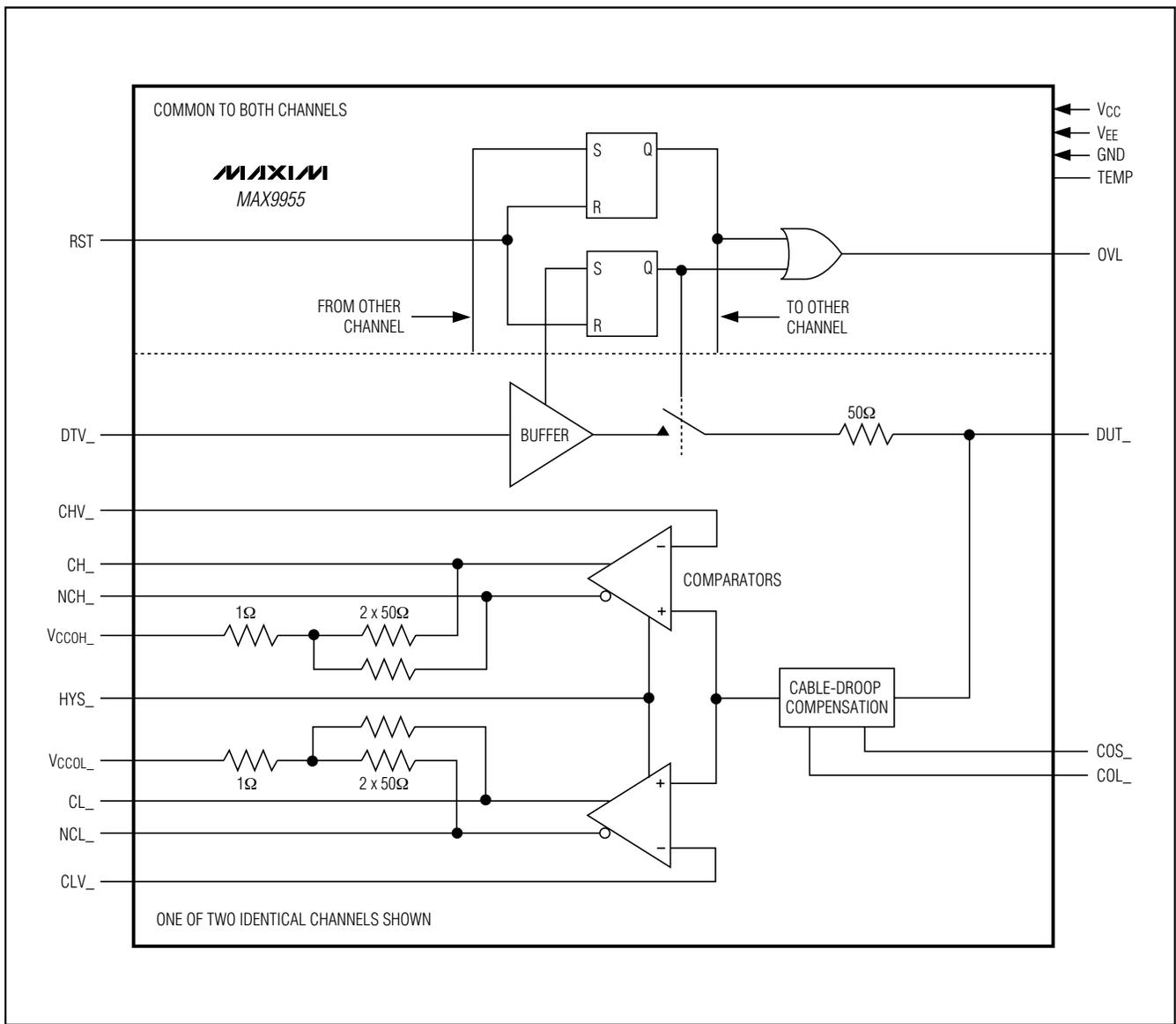
Figure 2. Functional Diagram
