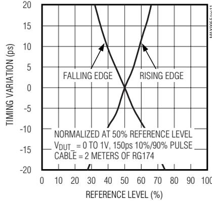
**COMPARATOR WAVEFORM TRACKING WITH CABLE COMPENSATION**
