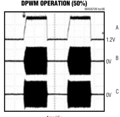
A:  $V_{CCV}$ , 200mV/div
