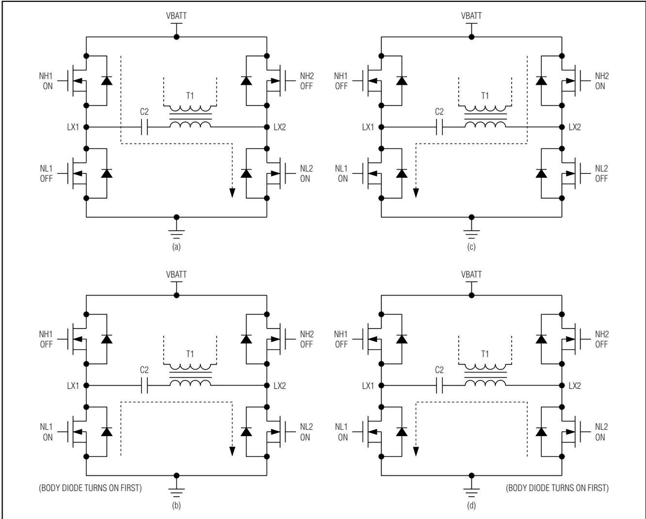
Figure 3. Resonant Operation
