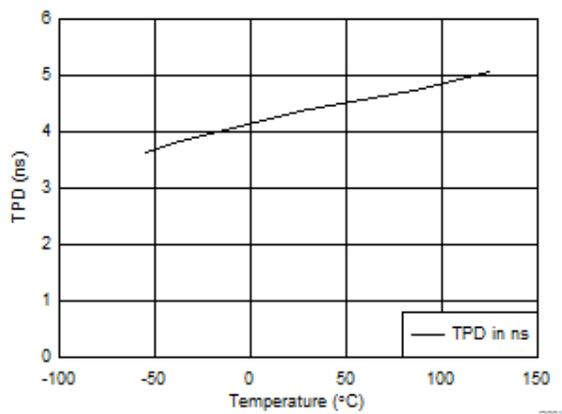
Figure 5-1. TPD vs Temperature at 5 V
