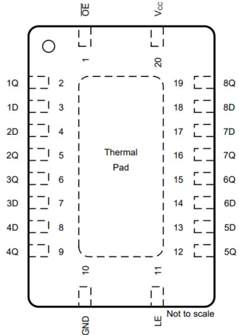
**Figure 4-2. RGY Package 20-Pin VQFN Top View**
