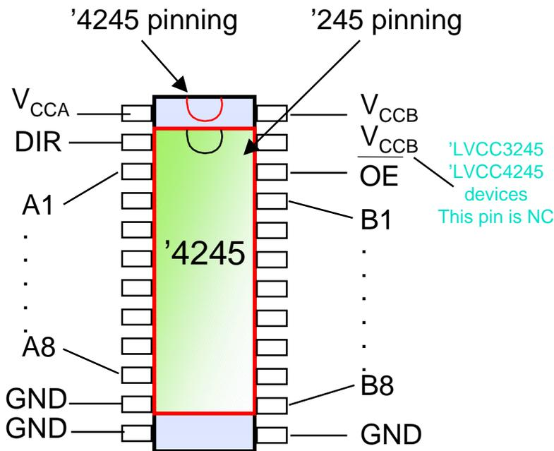
The 'ALVC164245 and 'LVC4245 have 5-V  $V_{CC}$  pins and 3.3-V  $V_{CC}$  pins.
