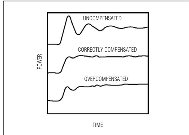
Figure 5. Laser Compensation
