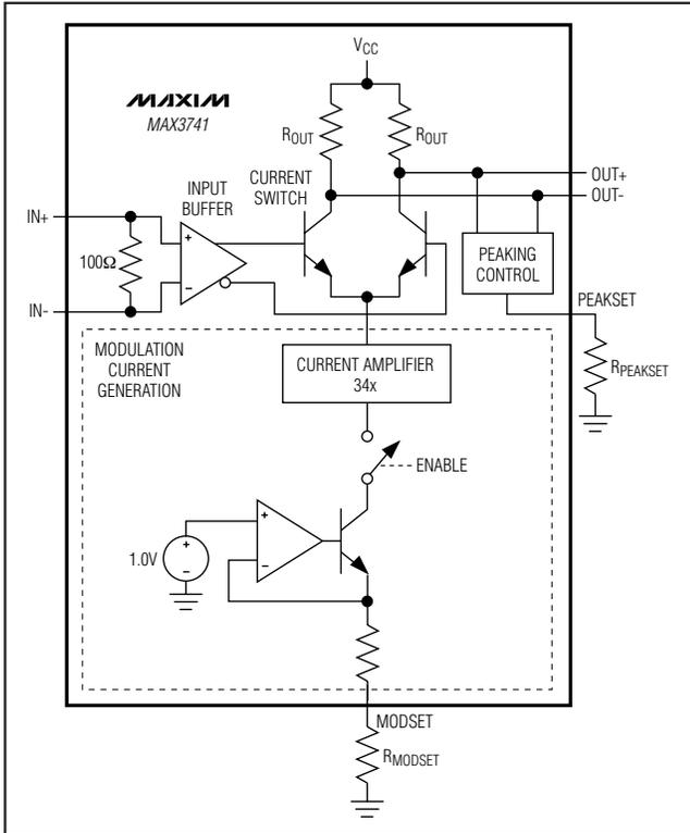
Figure 2. Modulation Circuit
